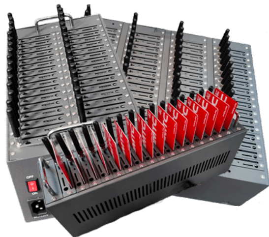
IMAGE 19. Example of sim-box used for running bot & troll farms
