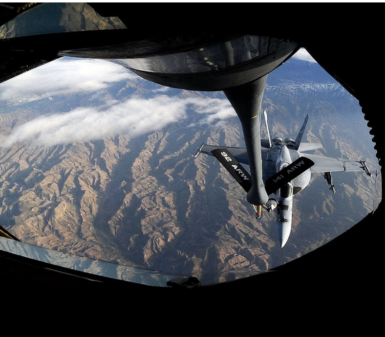
A US Navy F/A-18 Hornet Strikefighter receives fuel from a 22nd Expeditionary Air Refueling Squadron KC-135 Stratotanker over Afghanistan in 2010. IMAGE – US Air Force photo/Senior Airman Nichelle Anderson/release.
